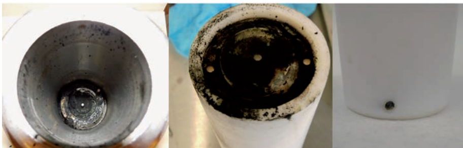
Fig. 2. Burnt out Teflon® cover from burning on the antenna during the ZnO NPs synthesis Source: IHPP PAS.
