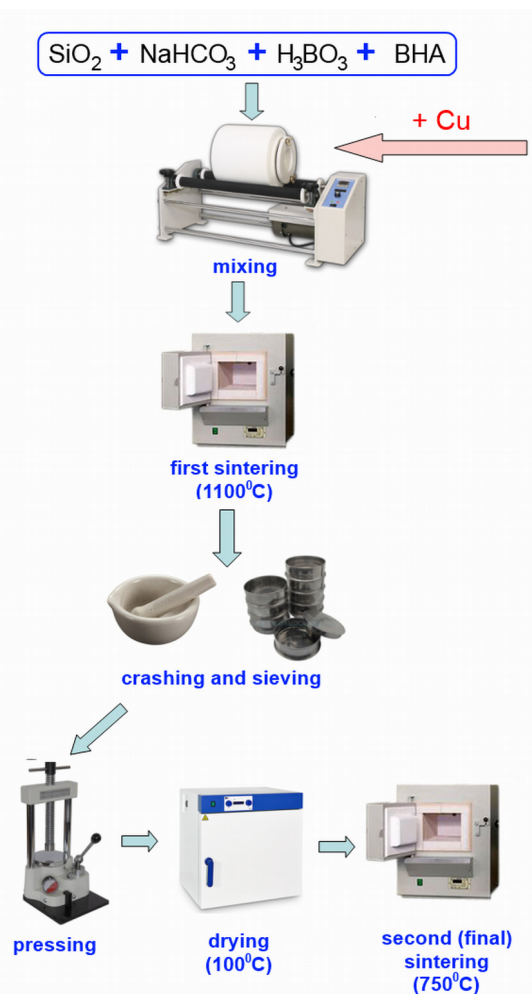
Fig. 2. Technological scheme of preparation of glass ceramic samples.
