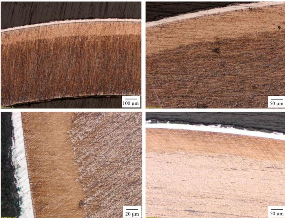
FIG. 144. Metallography images of sample IAEA-06 (PVD Cr coated Zr1Nb).
