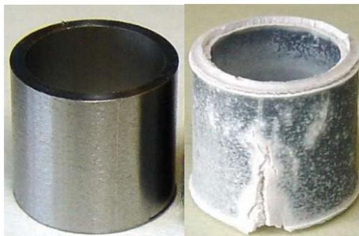
FIG. 132. Zr sample before (left) and after (right) oxidation in air at  $1200^\circ\text{C}$  for 2700 s with the normalized mass gain  $\Delta m/A=491 \text{ g/m}^2$ .
