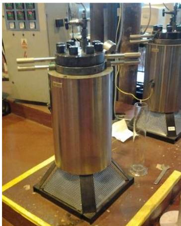
FIG. 10. Static autoclave used in the test.
