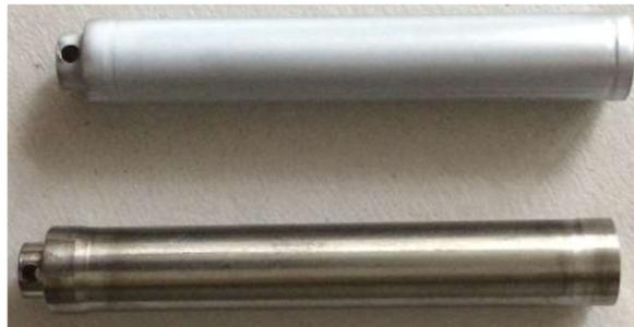
FIG. 127. Cr coated (top) and reference Zr (bottom) specimens.
