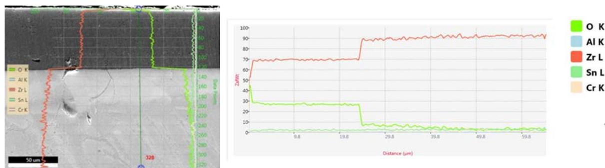
FIG. 98. The SEM-EDS line-scan over the oxide and  $\alpha$ -Zr layers in the specimen SPP 5 after exposure at 1200 °C / 30 min.
