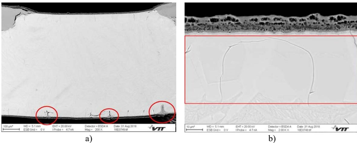
FIG. 101. Specimen SPP 6 after exposure at 1300°C / 5 min. a) Full cross section from the middle of specimen SPP 6, b) detail from the upper part shown in the left-hand side image.
