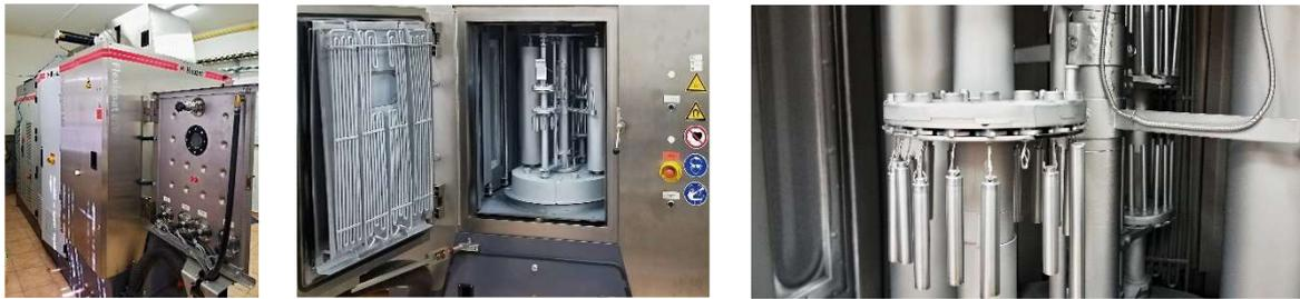
FIG. 2. Images of the Hauser Flexicoat 850 at CTU in Prague. Overview of the system (left); Deposition chamber (centre); Rotating sample holders with Cr target in the back (right) (Reproduced courtesy of Elsevier[182]).
